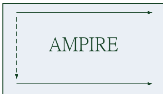
Fig. 1 Normal scan (pin 4, LR/UD = High or NC) Fig. 2 Reverse scan (pin 4, LR/UD = Low)
