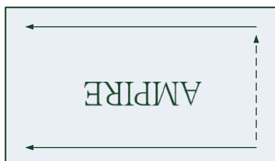
Fig. 1 Normal scan (pin 4, LR/UD = High or NC) Fig. 2 Reverse scan (pin 4, LR/UD = Low)
