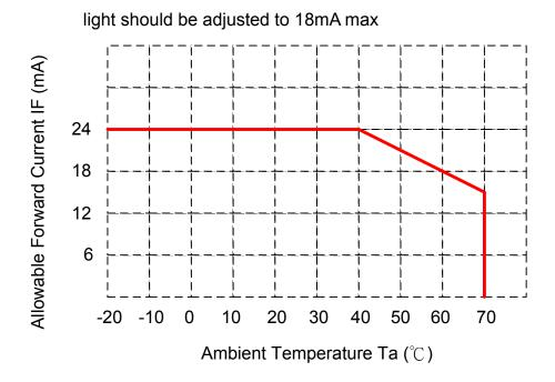
Note 4: When LCM is operated over 60°C ambient temperature, the IF of the LED back-
