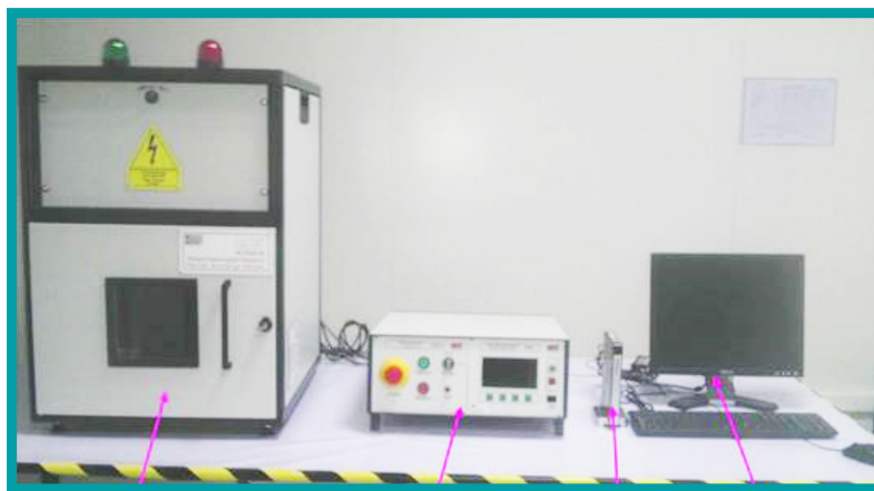
High Voltage Test Chamber PD Tester Computer
